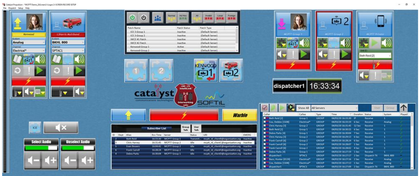
The Catalyst dispatch console can be used to establish LMR LTE interworking.
