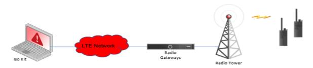
In a typical configuration, the Propulsion<sup>™</sup> Go Kit connects to an LTE Network with a Cradlepoint router for connectivity to Catalyst Radio Gateways.
