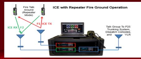
Digital Repeater Application – Enhancing Fire Ground Operations
