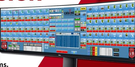
A strength of **Propulsion**<sup>™</sup> is the touch screen compatible, infinitely configurable user interface, which displays Unit ID, Emergency, and Call History. Dispatchers can simulselect or patch up to eight channels with intuitive graphical controls, instantly transmit on each module, uniquely set the volume for each module and differentiate audio on select and unselect speakers.
