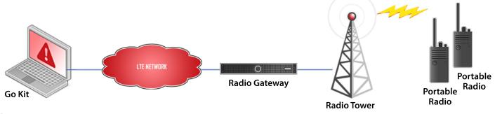
In a typical conffguration, the Propulsion™ Go Kit connects to an LTE Network with a Cradlepoint router for connectivity to Catalyst Radio Gateways.
