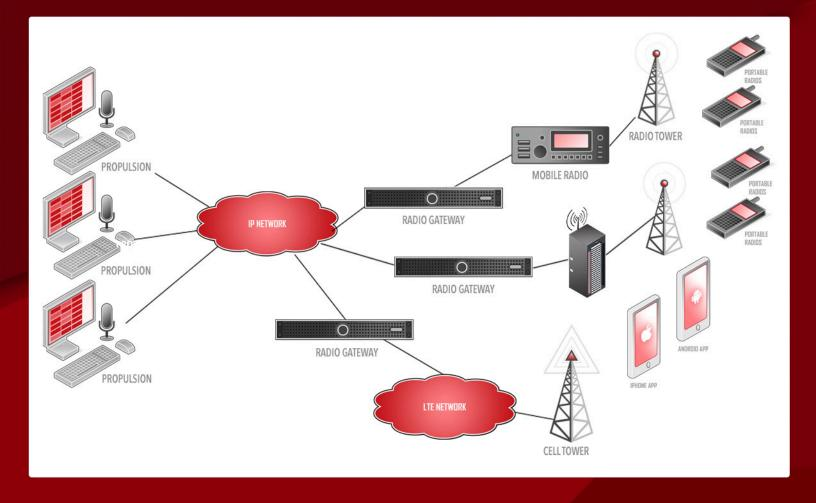
**Propulsion™** communicates over Internet Protocol (IP) based networks with radio Gateways that transmit and receive voice and control radio systems. These radio Gateways control the widest variety of radio resources in the industry:
