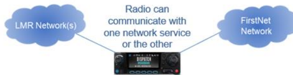
Figure 7 - Dual Mode Radios provide a communications interoperability function
